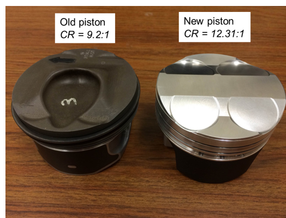
Figure C.1: Stock and new piston top designs [2]
